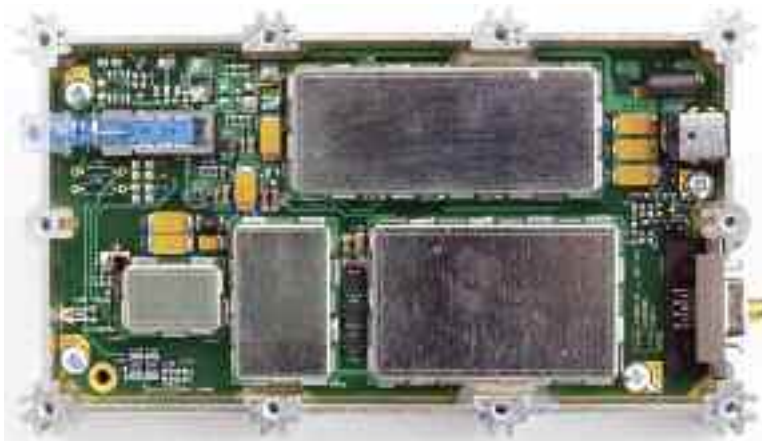
PHOTO 2: The receiver main printed circuit board.
