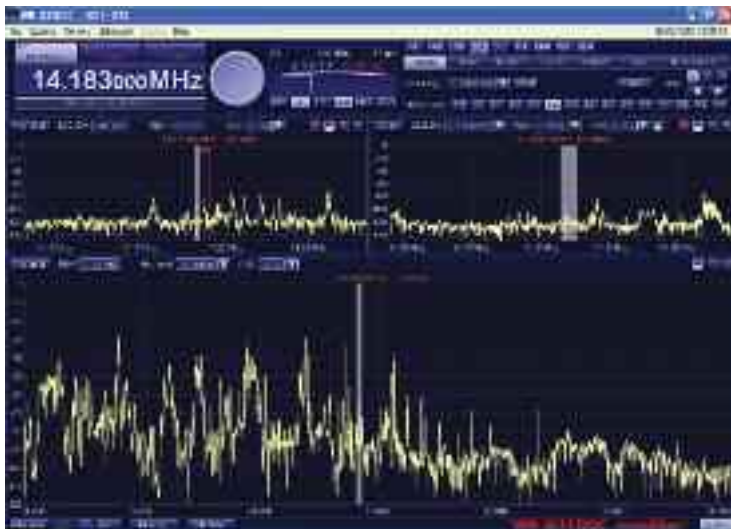
PHOTO 3: The control panel continuously displays three spectrum scans.
